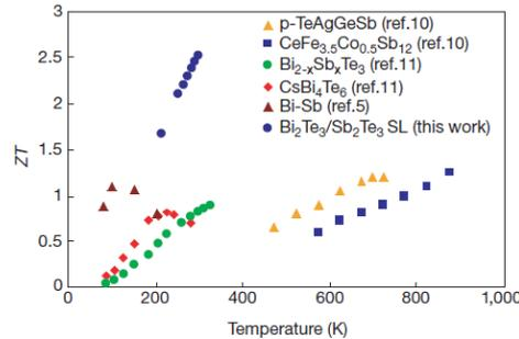
Figure 1: ZT-results of Venkatasubramanian et al. [1] in comparison with other thermoelectric materials without superlattice structure.(For mentioned references see [1].)
